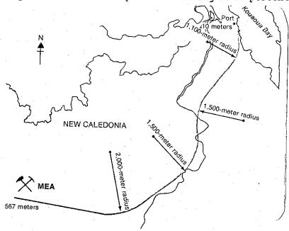
The same company which designed and installed the above system now have the capability to design belts operating under similar conditions with radii of horizontal curvature of 300 m.
