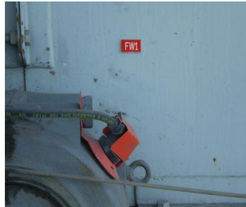
Figure 8. This sensor is used to monitor the bearing temperature
