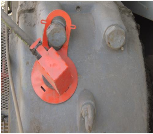
Figure 8. This sensor is used to monitor the bearing temperature
