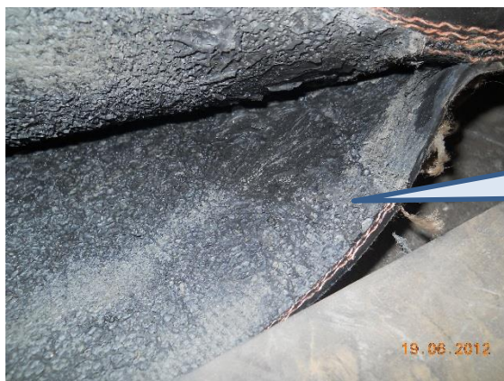
Figure 2. Results of under-curing
