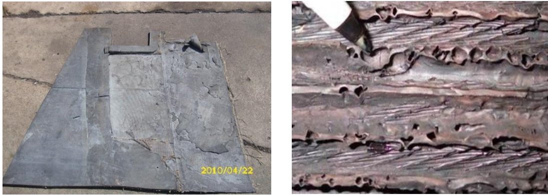
Figure 8. Result of insufficient pressure
