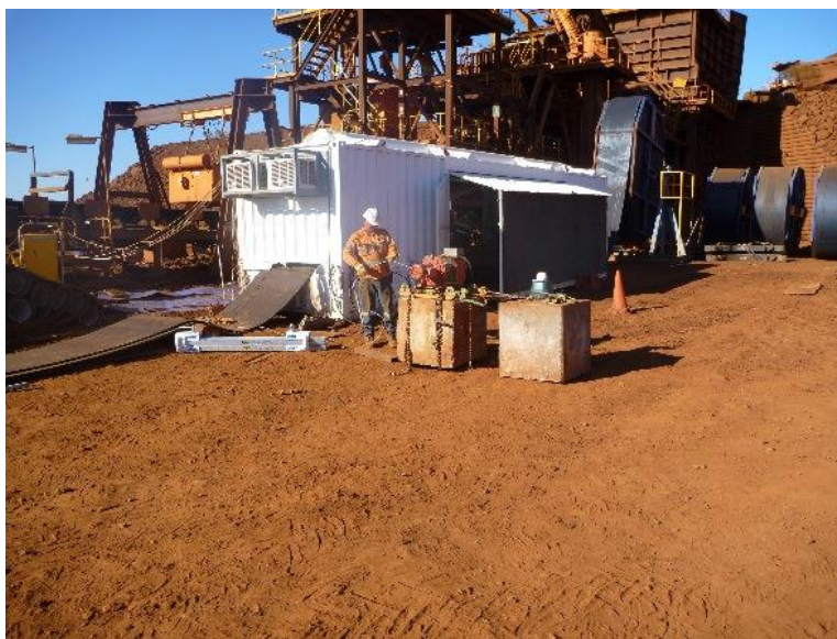
Figure 5. Example of a splicing container with temperature control
